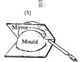
Run a knife around the edge of the mould and release the mirror.
