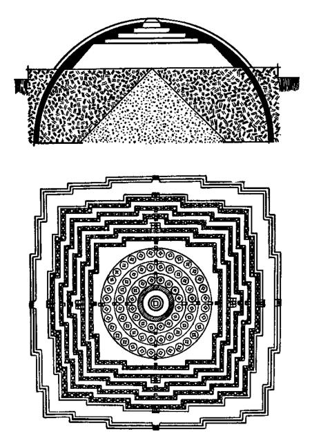
Borobudur temple. Elevation and ground-plan, illustrating the mandala pattern.
